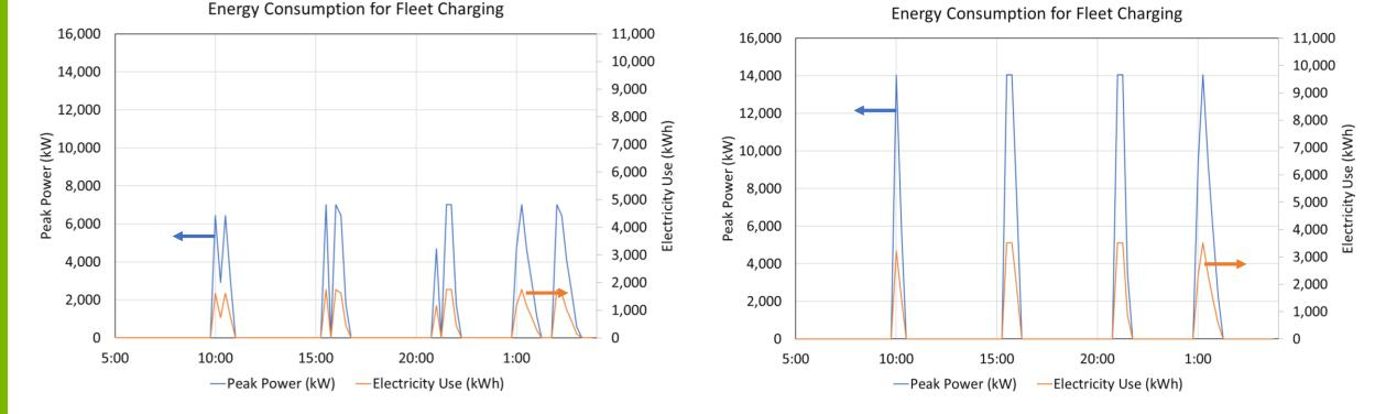
HEVISAM offers technoeconomic analysis of innovative charging solution by employing stationary Battery Energy Storage (BES) system that can offset the peak power during charging & reduce the cost of charging by lowering the demand charges.
